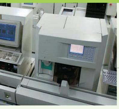
Sysmex's integrated hematology system mainly comprises hematology analyzers, instruments for making smear samples\* and the Laboratory Information System. In accordance with the order information, the test sample is automatically transferred to the various instrument, thereby contributing to the increased efficiency and speed of laboratory operations.
