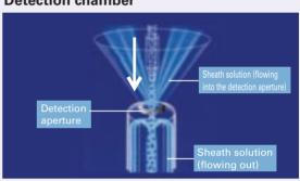
Passing cells one-by-one through the detection aperture
