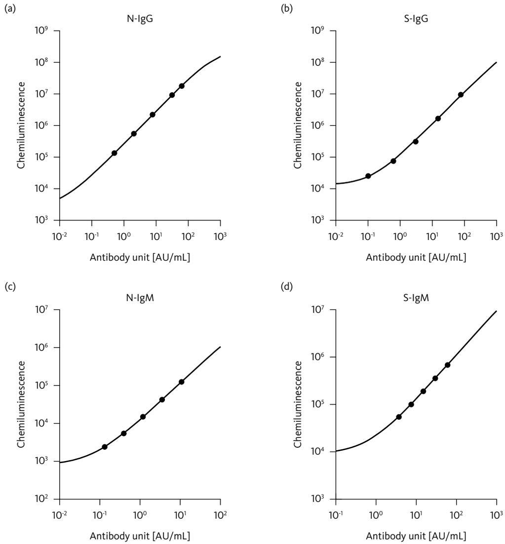
**Fig. 1** Relationship between chemiluminescence and the levels of each antibody. Working curve of *N-IgG* (a), *S-IgG* (b), *N-IgM* (c), and *S-IgM* (d).
