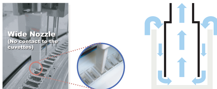
Fig. 14 Reaction cuvette WASH mechanism
