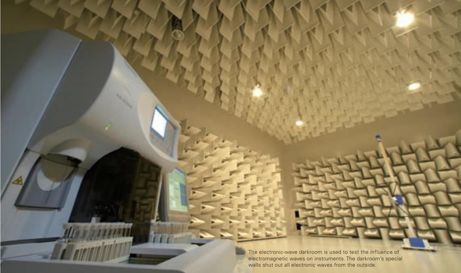
The electronic-wave darkroom is used to test the influence of electromagnetic waves on instruments. The darkroom's special walls shut out all electronic waves from the outside.
