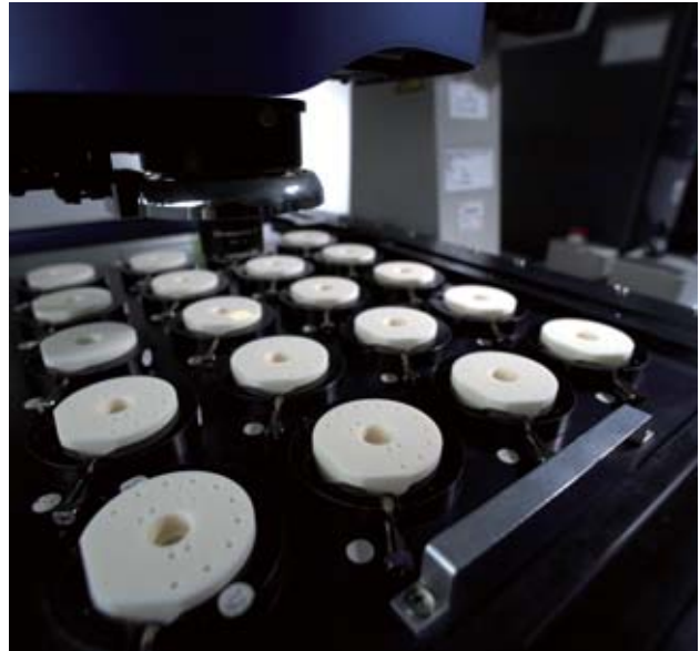
The sampling valve is an important component that is essential for accurately determining blood quantities. Sysmex manufactures these sampling valves, applying rigorous quality inspections to each one.
